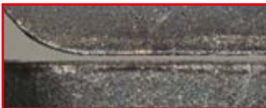
Cutting edge that is resistant to wear when machining ductile cast iron
