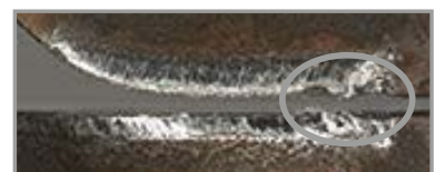
Chipped cutting edge
