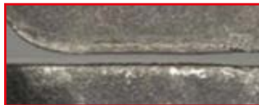
Cutting edge that is less susceptible to notching when machining stainless steel
