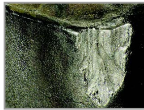
Fracture from welding chipping
